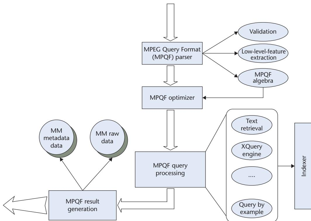
Figure 1. Architecture of MPEG Query Format-based retrieval engine.
